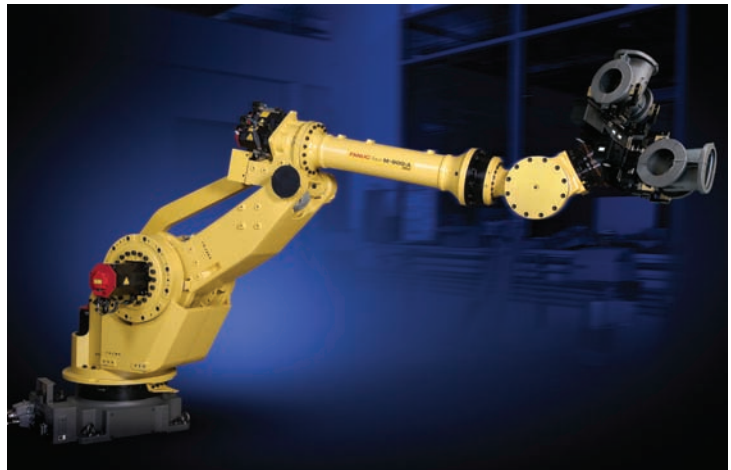
Cast iron valve body handling with M-900iA/350kg robot.
