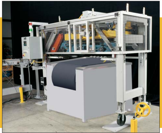
Guard in place
